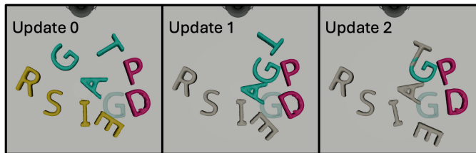
Fig. 11. Three iterations of the merged scene graph at various times during an episode of multi-object planar pushing (Sec V-B). Merged groups, shown with uniform colors, become more focused over iterations.
