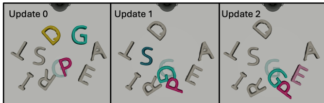
Fig. 10. Three iterations of the pruned scene graph at various times during an episode of multi-object planar pushing (Sec V-B). Pruned objects are shown in gray. Successive iterations refine the abstraction to adapt to failures, mistakes, or evolving environment states. Goal location for target "G" is overlaid.
